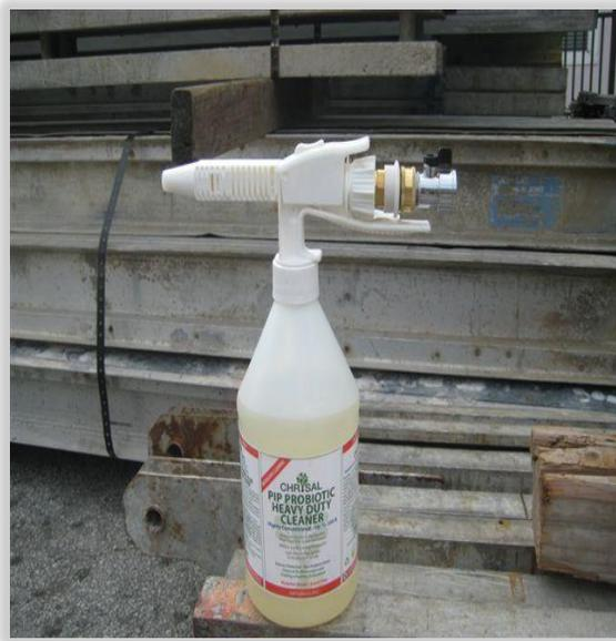
Inserting the quick disconnect into the foaming head
