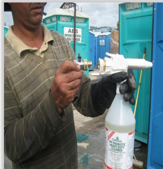
Attaching hose to foaming head with quick disconnect
